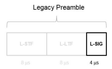
The L-SIG consists of one 4 µs symbol, which is a 3.2 µs OFDM symbol prepended with a 0.8 µs cyclic prefix. It contains packet information for the received configuration,
