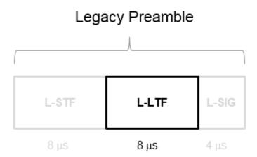
It is also the second field of the HT-mixed format preamble used in 802.11n and the VHT format preamble used in 802.11ac. Channel estimation, frequency offset estimation, and time synchronization rely on the L-LTF. The long OFDM training symbol consists of 53 subcarriers. IEEE Std 802.11-2012, Equation 18-8 and Equation 18-9 define the L-LTF.
