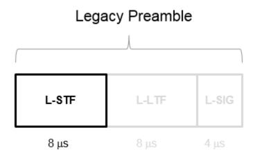
It is also the first field of the HT-mixed format preamble used in 802.11n and the VHT format preamble used in 802.11ac. The L-STF is 8 µs in length and consists of 10 repeated 0.8 µs symbols. Because the sequence has good correlation properties, it is used for start-of-packet detection, for coarse frequency correction, and for setting the AGC. The sequence uses 12 of the 52 subcarriers that are available in 20 MHz. IEEE Std 802.11-2012, Equation 18-6 and Equation 18-7 define the L-STF.
